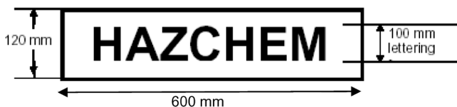
Figure 13.1 Form and dimensions of outer warning placard
