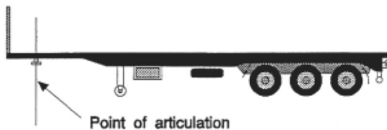
Point of articulation—kingpin for fifth wheel
