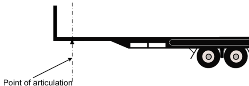
Point of articulation - kingpin for fifth wheel
